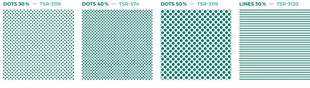
$^{1}\!/_{8}"$  (3.18 mm) diameter spaced  $^{9}\!/_{32}"$  (7.14 mm) centre to centre 30% coverage
